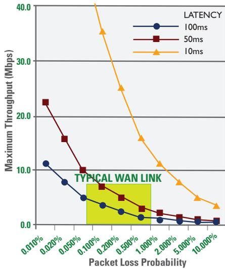
**Bandwidth, latency, and loss have a significant impact on effective throughput across the WAN.**
