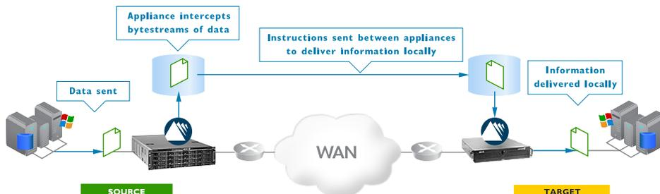
**Network Memory uses real-time byte-level deduplication to eliminate the transfer of repetitive data across the WAN.**
