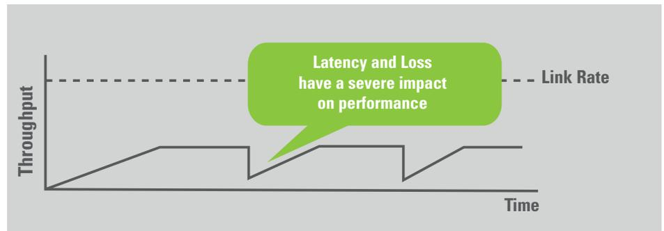
Periods of packet loss can have a “saw tooth” effect on WAN throughput, exacerbating the ill affects of latency.
